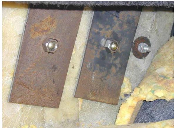
I've considered mounting a harness in this way and if you do the sums a plate of area 0.4m square is sufficient to withstand a 500Kg load ( big bloke with a 5G stop) with a fair bit of safety factor. so it should be fine, however as Pete says a roll-over bar should be considered before the harness. **350 matt**
