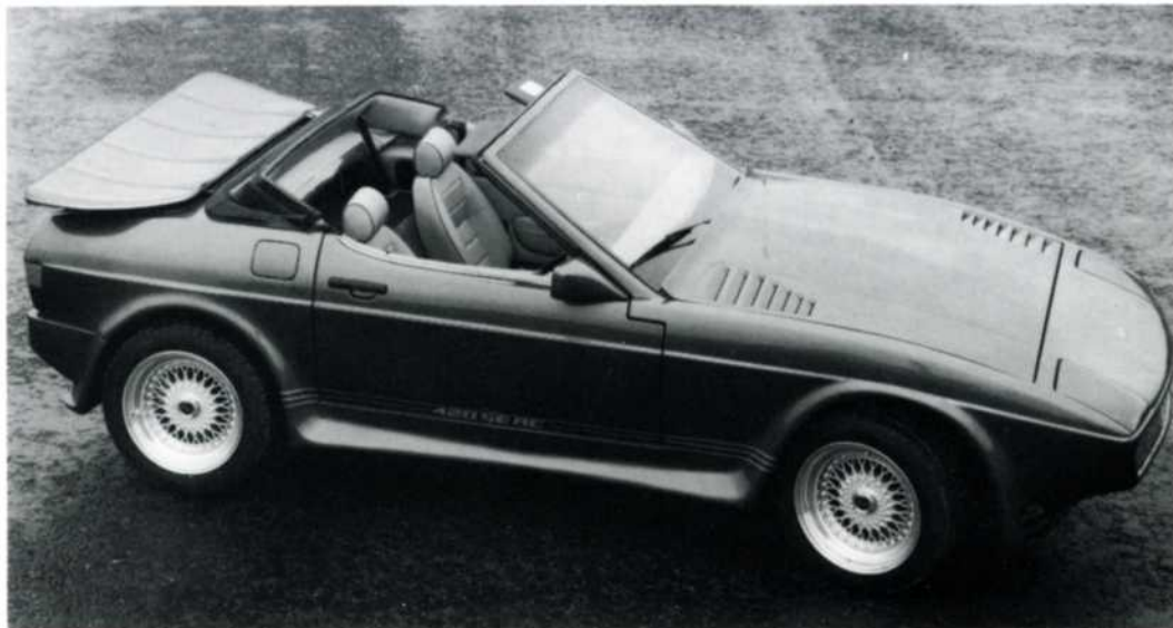
The 420SEAC model, officially put on sale in October 1986, had its body style developed in a factory-backed racing programme. Not only was the nose shorter and more rounded than that of the 390SE, but there were 'runningboards' along the side, and an aerofoil section behind the cockpit. (TVR)
