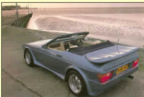
BONDED BODY: The sleek TVR shell is composed of Kevlar and carbon fibre which is light, but very strong.
